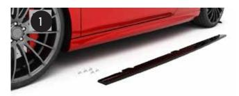
1. CHECK FITTING: Line up the diffuser and car side skirt.
